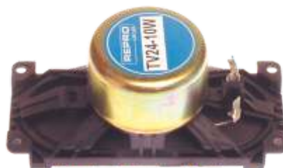
TV24-10W 2X4" 10W 14 ohms Distancia taladros 39x103 mm. Medida total 40x112 mm.
