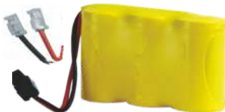
BAT238 (PT28) 3,6V/700 mA 1/2AAx3 Ni-MH d14,5x44x24 mm
