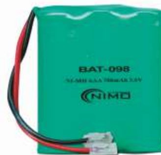
BAT098 3,6V/700 mA AAAx3 Ni-MH d11x33x45 mm.
